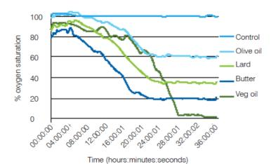
The above graph shows the degradation of different fats, oils and greases by BIOLOGIK BIO-BLOCK. As the substrates are degraded the % oxygen saturation decreases.
