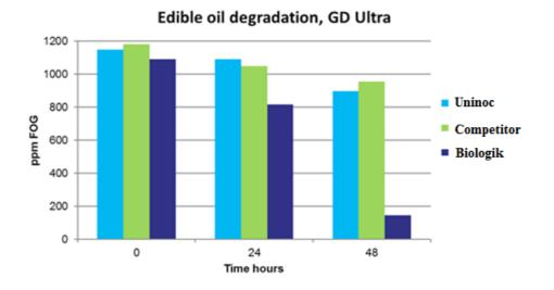
This graph show data collected using an Infra-Re d analyzer. This measures the actual oil concentration (including partial breakdown products such as fatty acids) before and after treatment.
